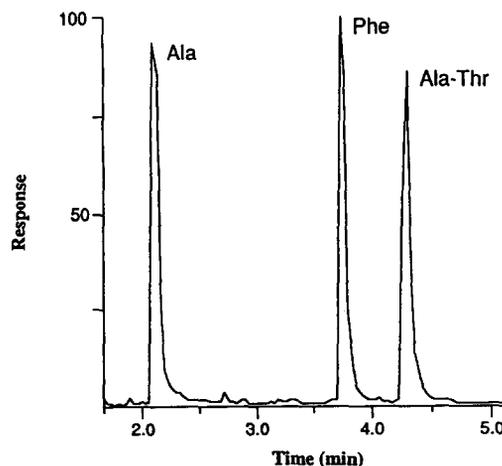
Fig. 2. Reconstructed ion chromatogram for derivatized Ala, Phe, and Ala-Thr analyzed by GC-NICI-MS using a wide mass range scan. GC conditions were as follows: column, DB-1 (15 m  $\times$  0.32 mm I.D.); injector, 280°C; splitless injection; column temperature, 150°C (1 min) to 190°C (1 min) at 10°/min to 250°C at 30°/min. Approximately 3 ng of each derivative was injected (based on the recovery of [ $^3\text{H}$ ]-Phe derivative).
