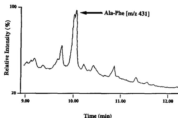
Fig. 5. Selected-ion chromatogram for 20 ng of Ala-Phe analyzed by GC-NICI-MS with selected-ion monitoring of  $[M - PFB]^-$ ;  $m/z$  431. GC conditions were as follows: column, DB-1 (15 m  $\times$  0.32 mm I.D.); injector, 280°C; splitless injection; column temperature, 75°C (1 min) to 175°C at 20°/min and then to 300°C at 10°/min.
